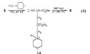
14 was isolated and redissolved in 50% (v/v) DMF-H<sub>2</sub>O solution, immediate evolution of CO<sub>2</sub> was observed. The workup of the reaction mixture provided 8 in 83% yield from 14. Similar results were obtained when isolated 14 was dissolved in 1 N guanidine hydrochloride solution; 8 was obtained in 62% yield from 14. When 5 was treated with formaldehyde-morpholine (pH 4.5) and 14 was not
